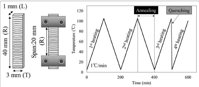
Fig. 1 Schematic diagram of the sample attached to the forced-vibration dynamic viscoelastometer and temperature program for measurement of temperature dependence
