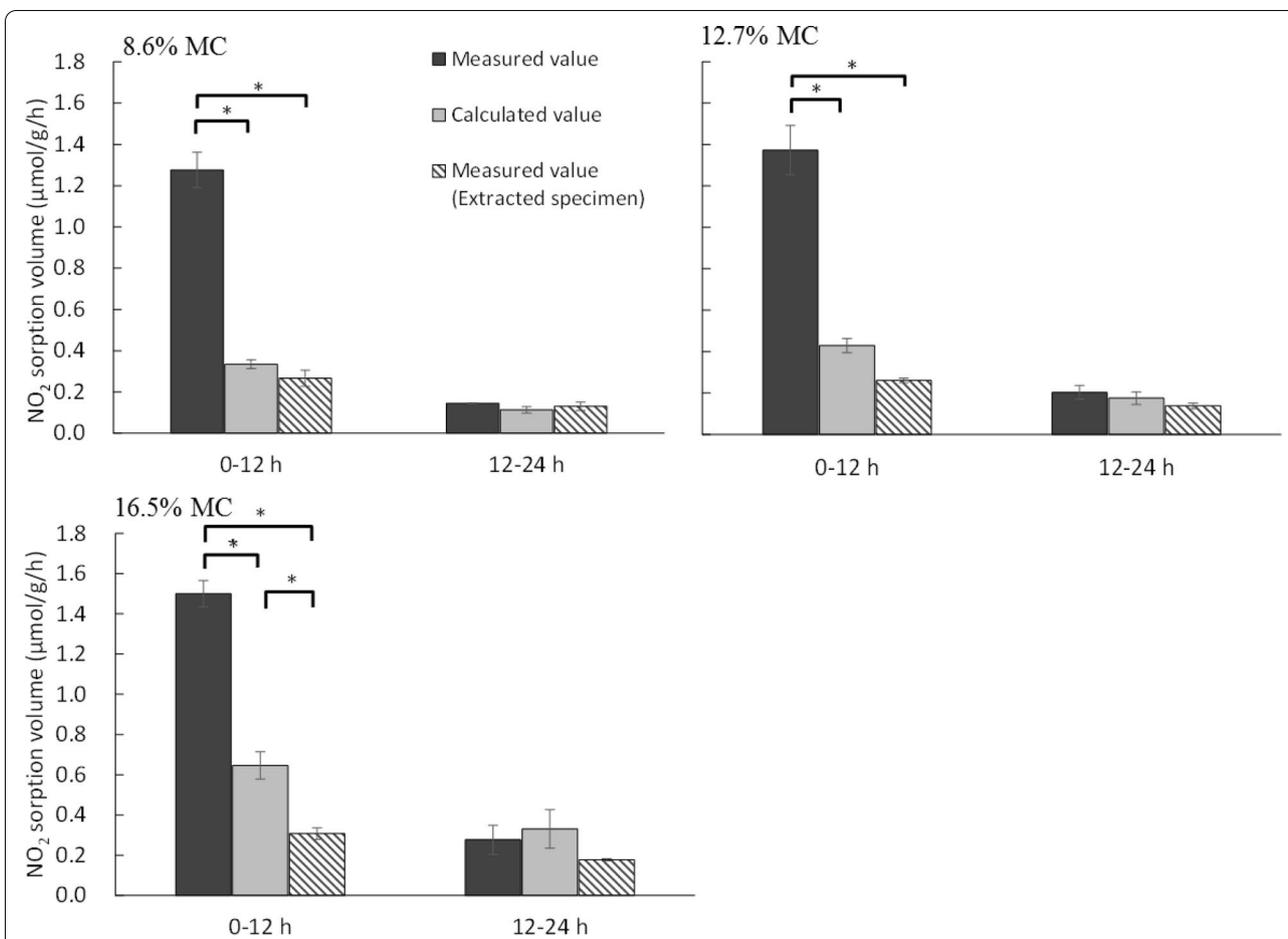
**Fig. 8** NO<sub>2</sub> sorption volume per unit weight and time from 0 to 12 h (0–12 h) and from 12 to 24 h (12–24 h), given as measured values [ $Q_{WNO_2}$ ] and calculated value. The error bars show the standard deviation ( $n=3$ ). \*\*:0.01 >  $p$  (Tukey method)
