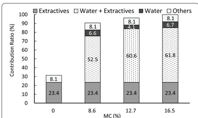
**Fig. 9** Contribution ratios of water only, extractives only, water + extractives, and others with respect to NO<sub>2</sub> sorption under different MC conditions. The ratio for each MC condition shows the ratio of its value to the value under the 16.5% MC condition
