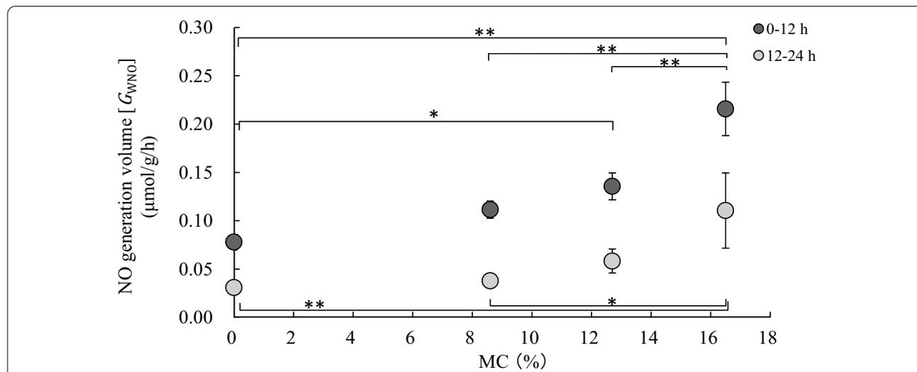
**Fig. 5** NO generation volume per unit weight and time (0–12 h and 12–24 h),  $G_{\text{WNO}}$ , with different MCs. The error bars show the standard deviation ( $n = 3$ ).  $*: 0.05 > p, **: 0.01 > p$  (Tukey method)
