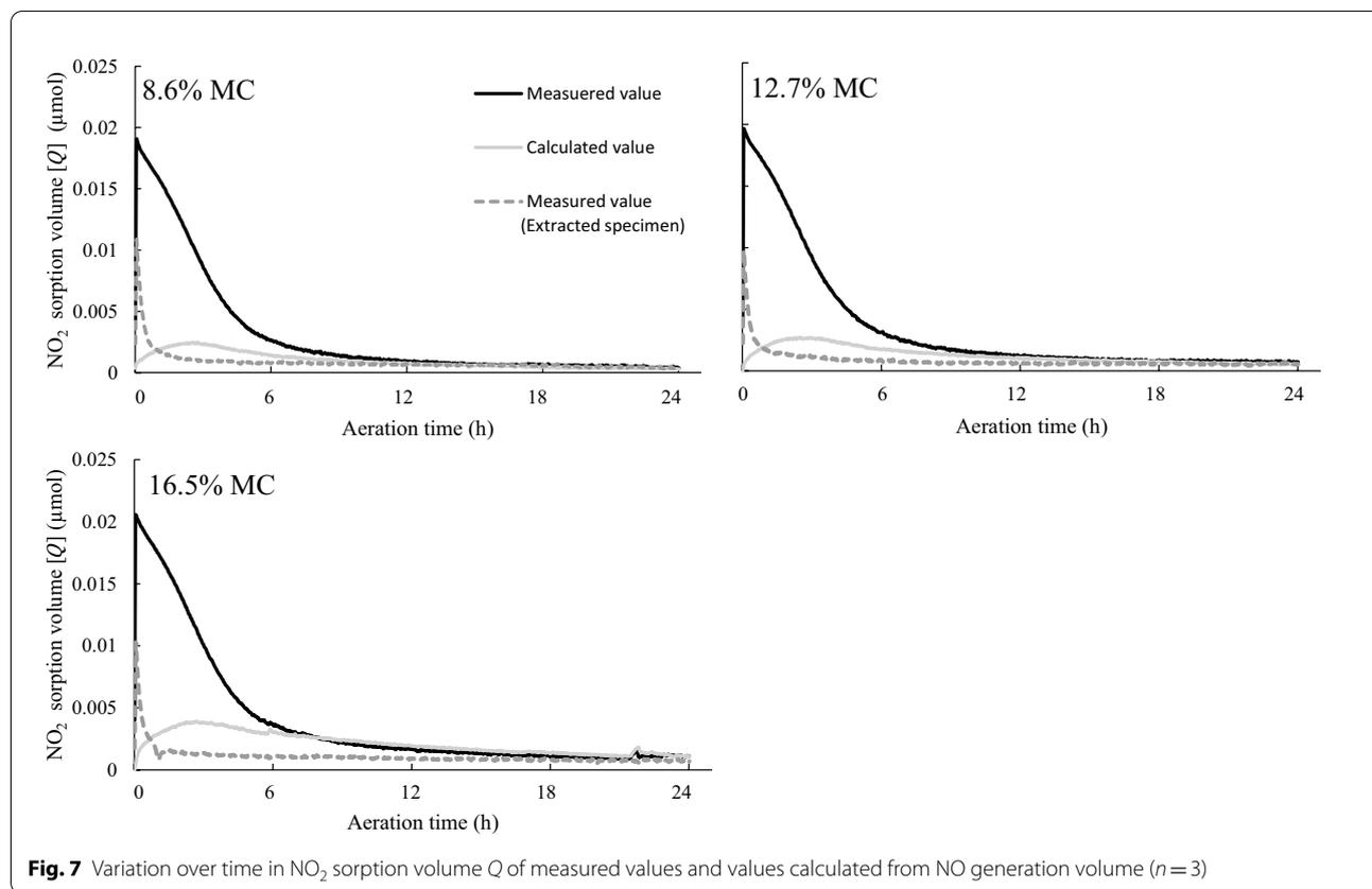
$$\text{Contribution ratio of extractives only (\%)} = \frac{(Q_{WNO_2} \text{ of non-extracted specimen}) - (Q_{WNO_2} \text{ of extracted specimen})}{(Q_{WNO_2} \text{ of non-extracted specimen at 16.5\% MC})} \times 100.$$
