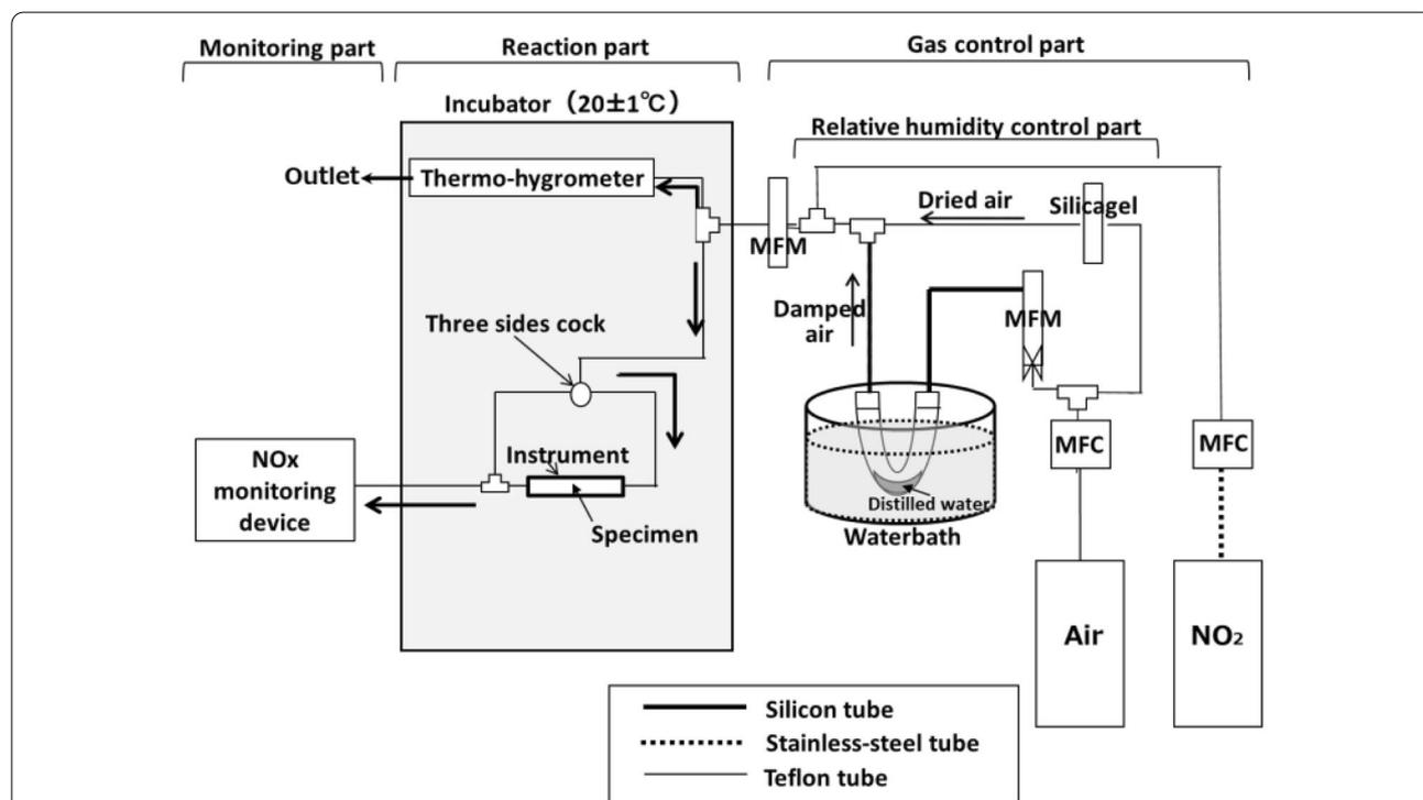
**Fig. 1** Experimental system for NO<sub>2</sub> sorption test. MFC refers to the mass flow controller which controls the flow rate. MFM refers to the mass flow meter which monitors the flow rate
