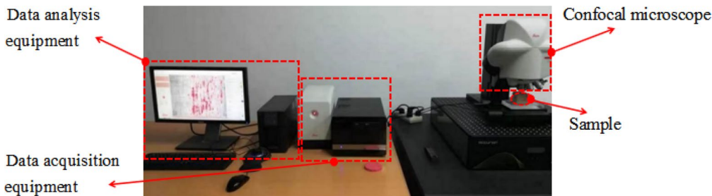
Fig. 8 The scanning system of Leica 3D confocal microscope
