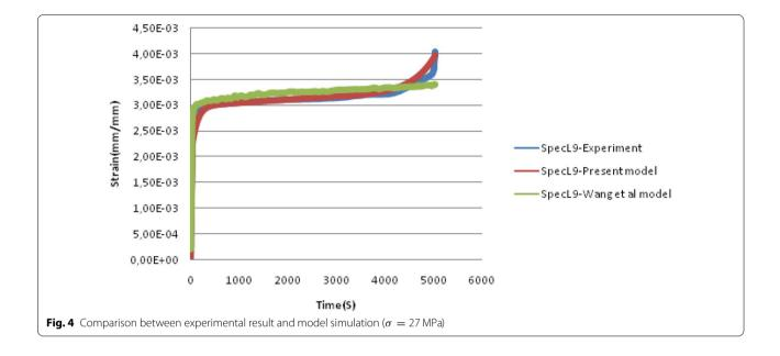
The following figures (Figs. 3, 4 and 5) show the comparison between the experimental creep curves and the curves calculated from the model.
