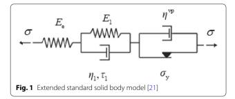
approaches for the description of this phenomenon. Authors such as Wang, Cai, Pierce et al. [13, 15, 16] have modified the components of the model by introducing a damage variable to explain tertiary creep.
